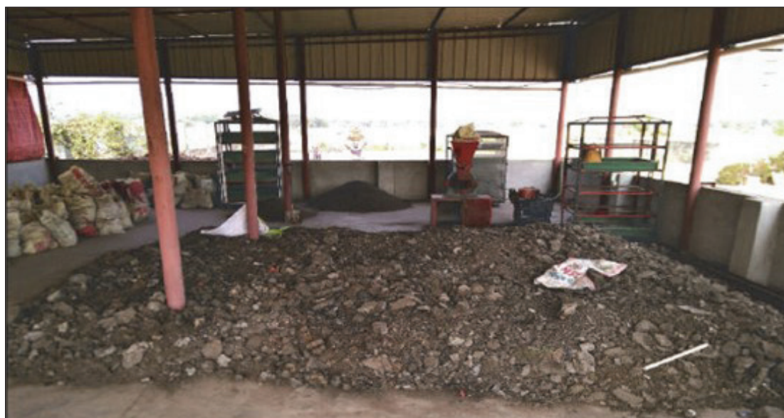
Figure 4.32: Preparation of the Dewatered Sludge Cakes in Faridpur, Bangladesh, Prior to Transportation to the Nearby Co-composting Plant
